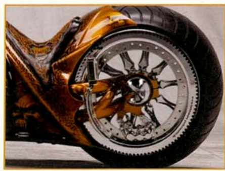
Concealing the mounting bolts for the pulley and rim brake was one of the hardest parts of the build
